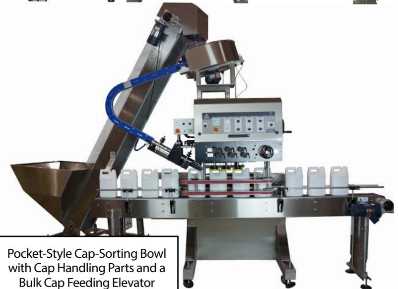
Pocket-Style Cap-Sorting Bowl with Cap Handling Parts and a Bulk Cap Feeding Elevator
